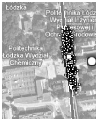
Fig. 10. A screenshot of the particle filtering simulation: large round dot – GPS location readout, large square – estimated user location, small squares – particles. Note that the algorithm eliminates the particles that would enter forbidden areas (i.e. buildings, fences, etc.).
